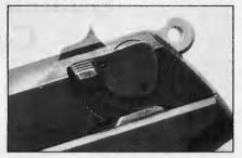
ABOVE: An ambidextrous hammer-drop safety lever is mounted to the P-85's slide.
